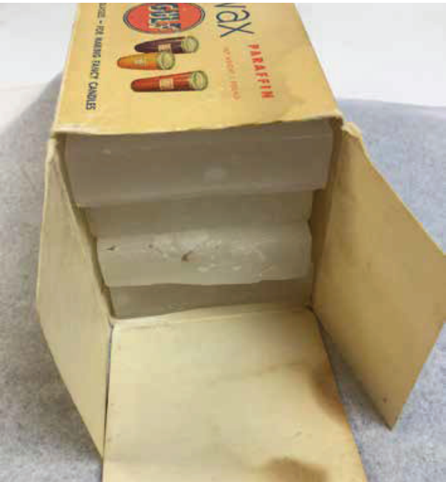
Fig. 1. NMR was first seen in this resonant cavity, filled with paraffin obtained from the First National Store on Purcell’s way to work. (leftover wax in original box courtesy of Pound)
