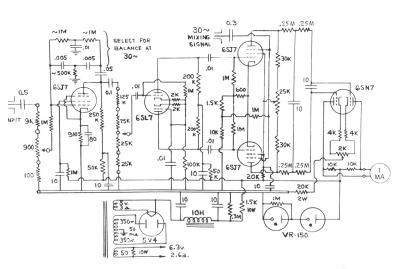
Figure 3: Nowadays you just buy a lock-in amplifier, or do the equivalent thing with software operating on digitized data. But in 1950 you built your own equipment, as Ewen did with his 8-tube circuit (from his thesis). Circuit mayens will raise an eyebrow at the component values of the two-stage RC low-pass filter preceding the 6SN7 differential output stage.
