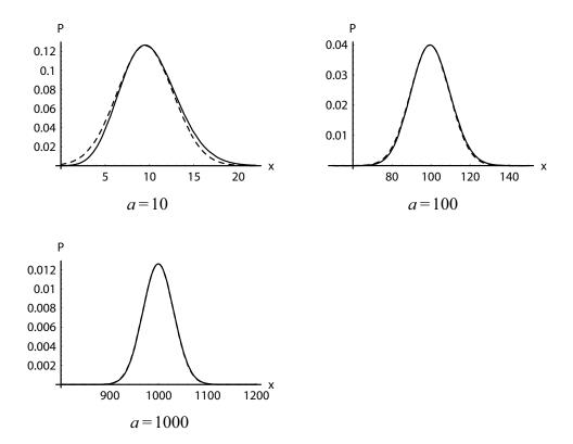
We should check that the Gaussian probability distribution in eq. (7) has an integral equal to 1. In doing this, we can let the integral run from  $-\infty$  to  $\infty$  with negligible error. Using the general result,  $\int_{-\infty}^{\infty} e^{-y^2/b} dy = \sqrt{\pi b}$ , and letting  $b \equiv 2a$ , we see that the integral is indeed equal to 1.
