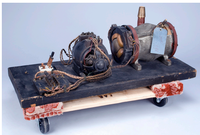
Figure 6: Vacuum technology circa 1920: the Holweck pump [Reproduced with permission from CHSI]
