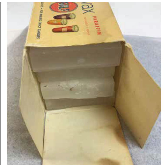
Fig. 1. NMR was first seen in this resonant cavity, filled with paraffin obtained from the First National Store on Purcell’s way to work. (leftover wax in original box courtesy of Pound)
