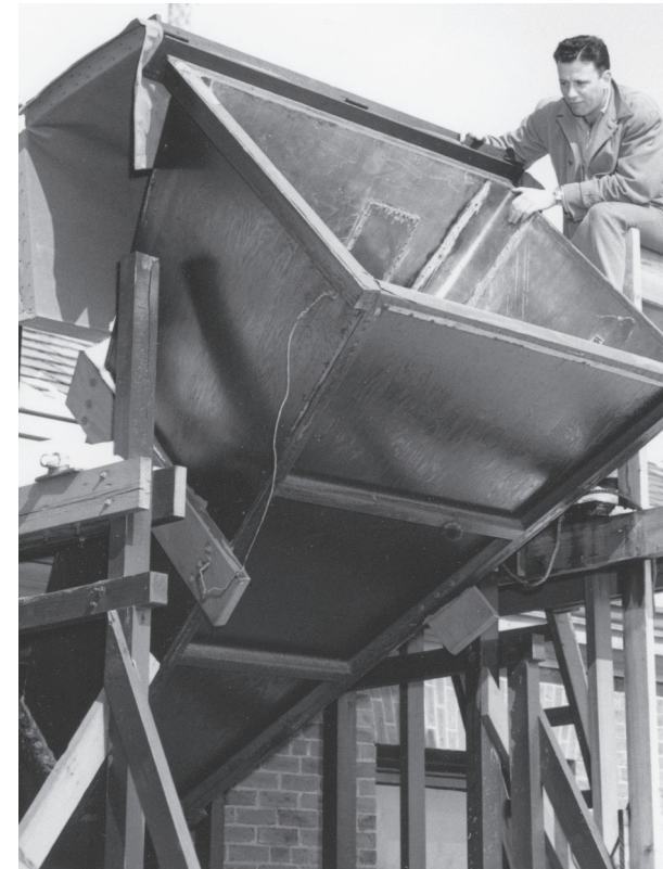
Figure 1: Harold "Doc" Ewen provides scale for the 1420MHz horn antenna, made from copper-clad plywood, on the parapet outside Lyman 4th floor. The canvas cover was added after the horn funneled a rainstorm into the lab (which Ewen remarked was his first "signal from space").
