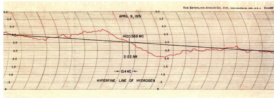
**Figure 4:** The galactic hydrogen emission signal at 1420MHz (21cm), as traced in red on the strip-chart recorder two weeks after its discovery. The frequency-switched modulation technique causes the trace to have a differentiated S-shape. The sloping black line approximates the receiver's drift over the 20-minute observation. (Reproduced from Figure 18 of Ewen's 1951 thesis.)
